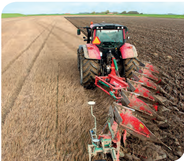
On-land ploughing with high accuracy using TWIN steering. GPS antenna will turn when the plough turns.
