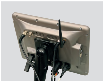
Rugged magnesium alloy enclosure
