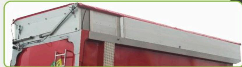
Aluminium extension sides with pneumatic PVC cover
