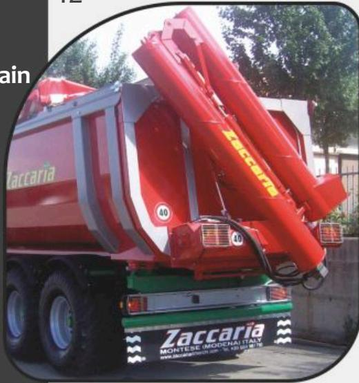
The system consists of a horizontal scroll and a vertical scroll hydraulically operated by self gear pump with cardan shaft and distributor with electric activation through pushbutton located in the cab. Closing window with hydraulic activation operated by tractor distributor. Easy disassembly of scroll system.
