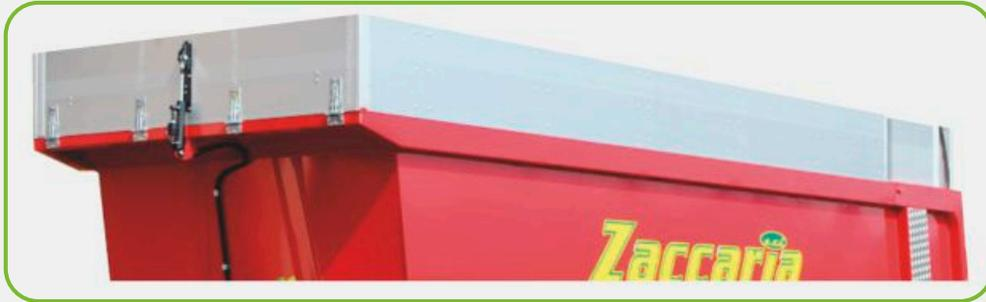
On demand: Aluminium extension side and hydraulic opening of the front extension side.
