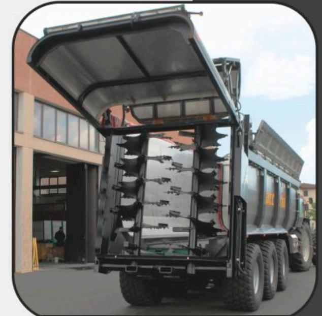
Manure spreading module on two big rollers interchangeable with door with hydraulic opening
