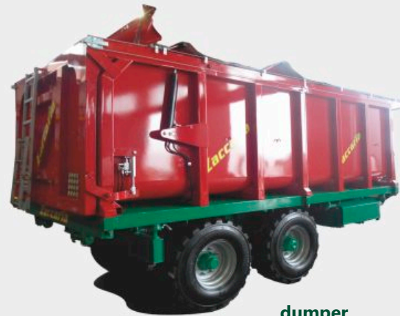
dumper with lateral parking stand
