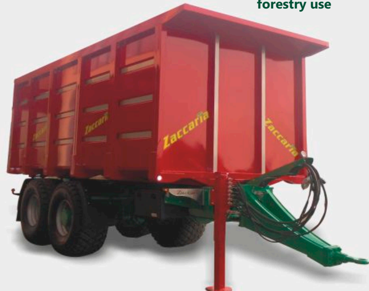
Trailers with dumper for forestry use
